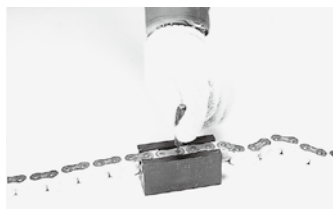
Figure 16: Disconnecting Poly Steel Chain
