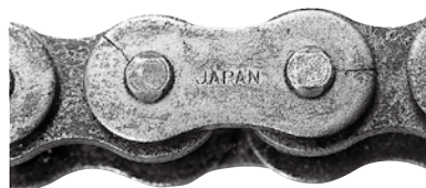
Hydrogen embrittlement cracking
