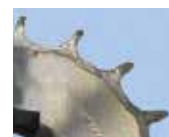
Standard stainless steel sprocket after use
